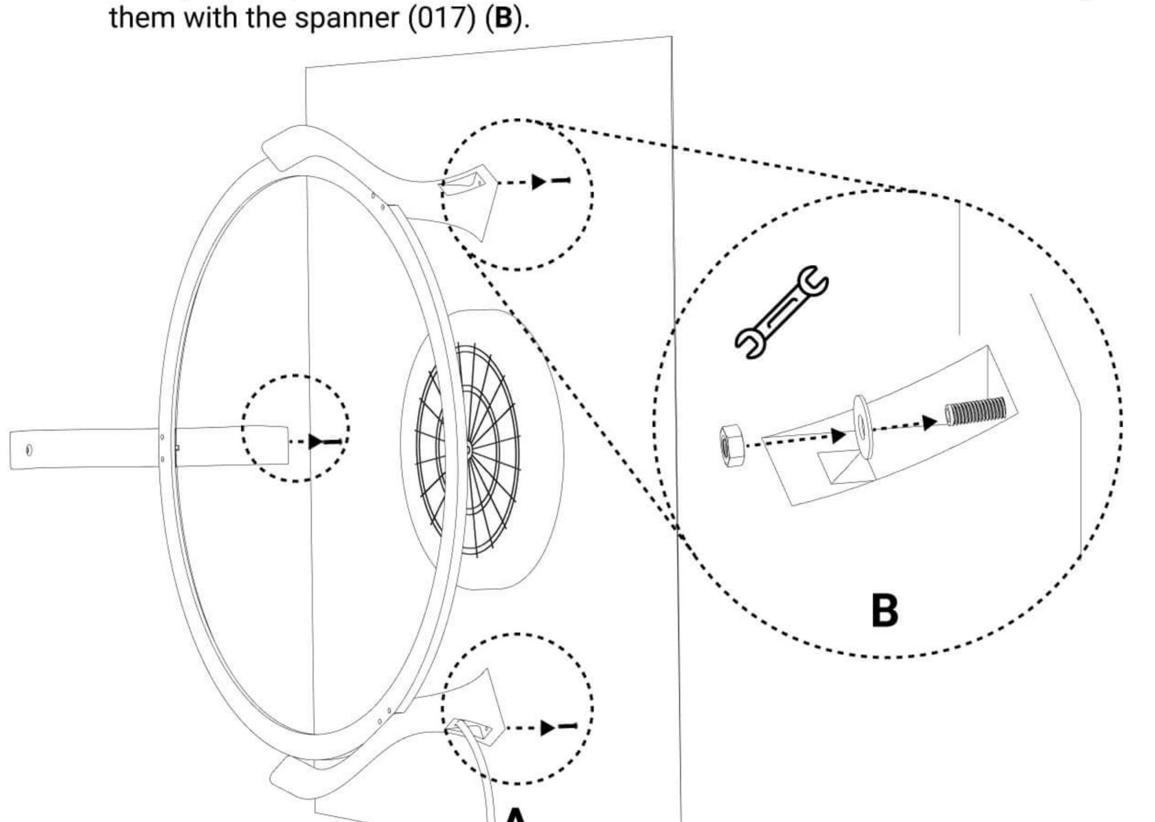
Determine the appropriate place for the processing unit. Make sure the cables of
